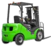
3.0T FORKLIFT 3m Duplex Mast, Pneumatic Tyres
