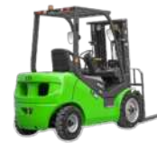
3.5T FORKLIFT 3m Duplex Mast, Pneumatic Tyres
